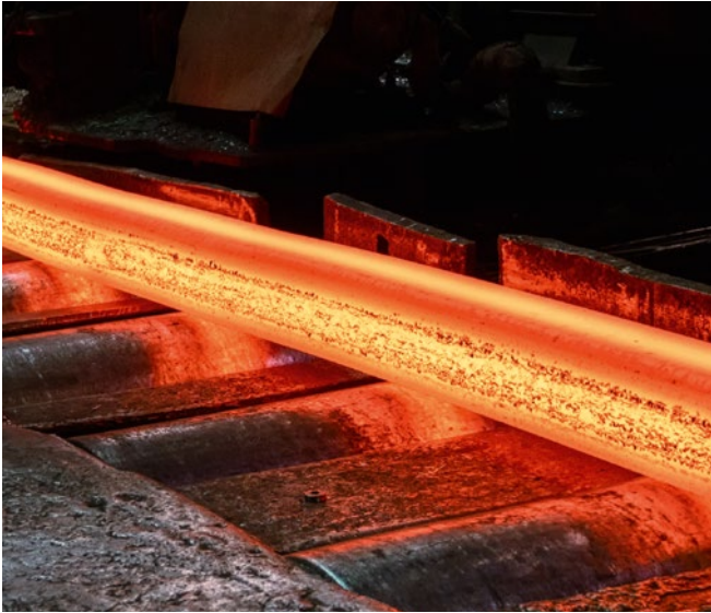
Scale and oxide significantly change the radiation properties
