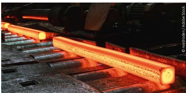
Scale and oxide significantly change the radiation properties
