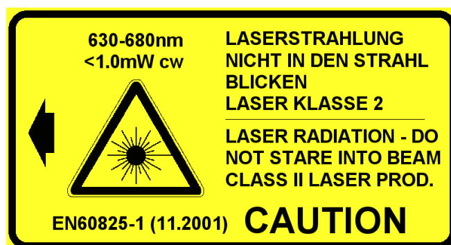
Fig. 5.2 Laser warning label affixed to the pyrometer
