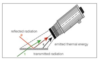
**Fig. 2** Composition of radiation received by the pyrometer's sensor.
