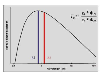
**Fig. 2** Two-colour pyrometers detect radiation at two wavelengths and produce a temperature reading based on the ratio of these intensities.
