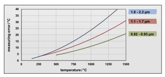
**Fig. 8** Measurement error of single-wavelength pyrometers with different wavelength when emissivity changes by 10 %
