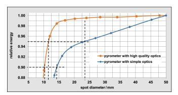
**Fig. 6** Comparison of the SSE curves of two pyrometers with high quality and simple optics
