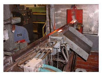
Fig. 1 Billet rejection based on temperature
