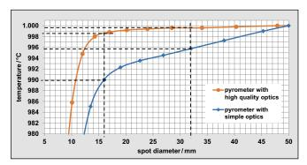
Fig. 5 The effect of target object size on the temperature reading
