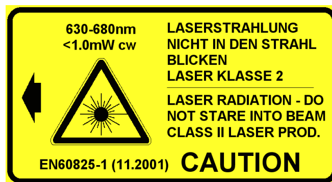
Fig. 1.2 Laser warning label affixed to the pyrometer
