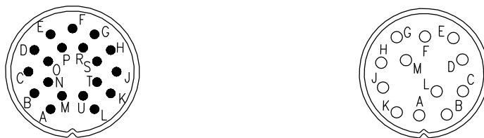
Pin layouts (PZ 20/X exterior view): 19-pin flange plug and 12-pin socket (Binder Series 723)
