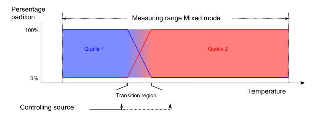
Two signal sources are linked in the instrument in mixed mode. Only source 1 is transmitted for the lower temperature range and only source 2 for the higher temperature range. Both sources are weighted on a percentage basis in the transition area which is defined by the transition start and end temperatures. The "controlling source" checks whether the working point is below, within, or above the transition area.
