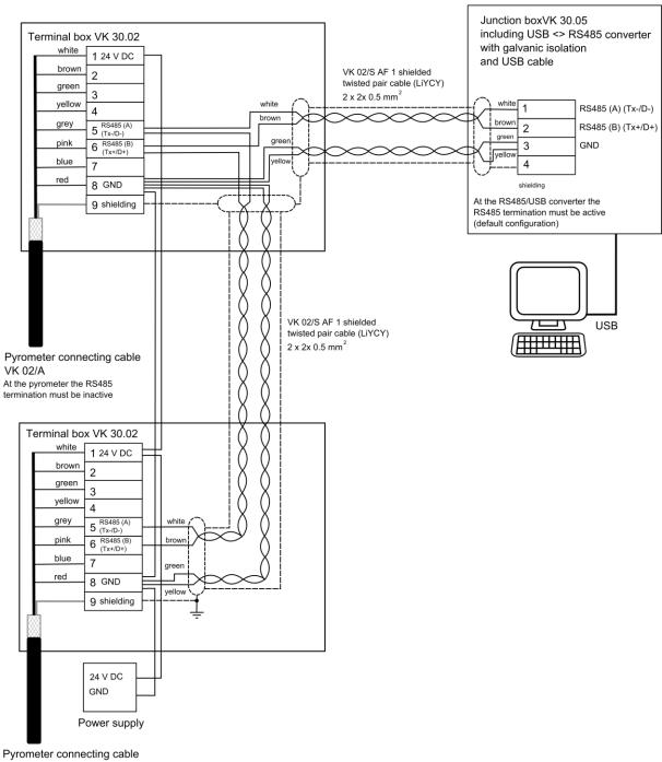
Pyrometer connecting cable VK 02/A
