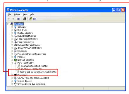
Ports (COM and LPT). You will see a listing of ports and should now be able to see which COM Port the PA USB connection assigned to. The PA USB connection will be indicated as a USB-to-Serial Comm Port. In this example, COM Port 5 has been assigned to the adapter. You will need to select this particular COM Port in the software settings.
