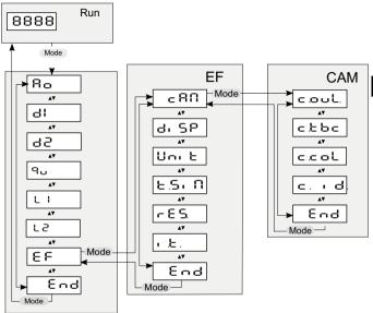
CAM Parameter and submenu only available at pyrometer with camera.
