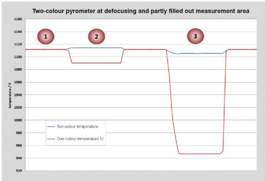
**Fig. 6** Influence of the measuring distance on the two-colour and spectral temperatures.
