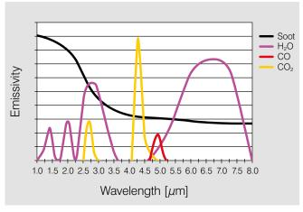
Fig. 2 Radiation characteristics of combustion gas
