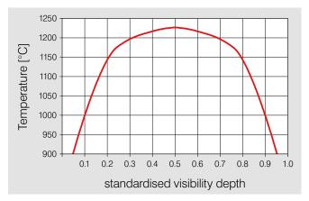
Fig. 4 Temperature distribution inside the combustion chamber
