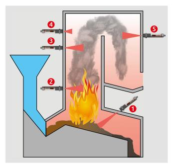
Fig. 1 Pyrometric measuring locations in an incineration plant 1: Firebed, 2: Flame, 3: Exhaust gas inside the furnace, 4: Exhaust gas in the area close to the wall, 5: Exhaust gas after the last supply of combustion gas
