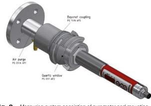
Fig. 3 Measuring system consisting of pyrometer and mounting with bayonet locking, quartz glass and purging air nozzle
