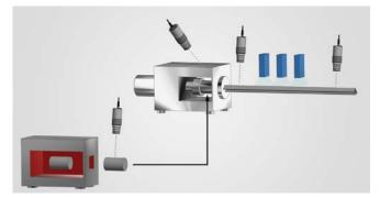
Fig. 1 Pyrometric temperature measurement at the extruder outlet.
