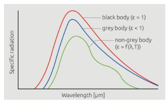
Fig. 2 With aluminium, the emission is wavelength-dependent (non-grey body).
