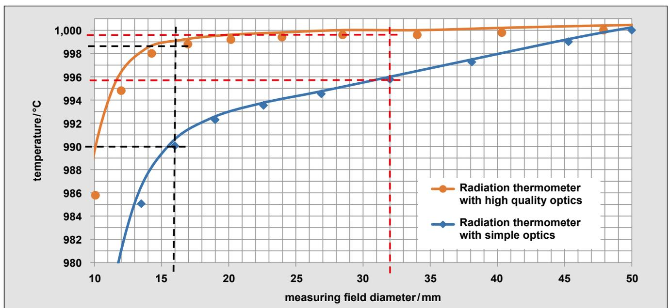
**Picture 8** Effects of a changing target size on the temperature.
