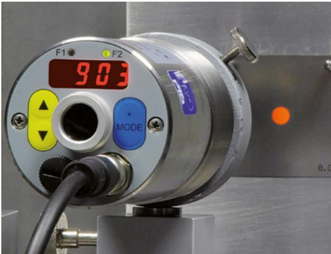
**Picture 4** Determining the optical properties of a radiation thermometer.
