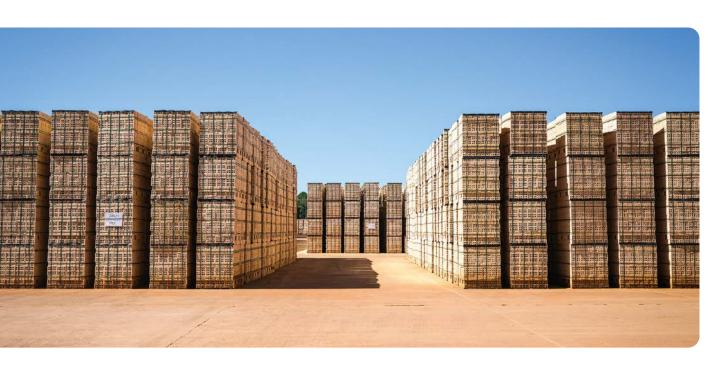
Working time: \_\_\_\_\_ 50 weeks per year 6.5 days per week 2 shifts per day 10.8 hours per shift (effective) Reference size: \_\_\_\_\_ 222 mm x 106 mm x 73 mm - 2.3 kg (fired) 105,000,000 bricks per year Output - reference size: Plant data: 2.2 kg/dm<sup>3</sup> Density: Preparation water content: 22.4 % 10.6 % Loss on ignition: 40.3 hours Drying time: 43.0 hours Firing time:
