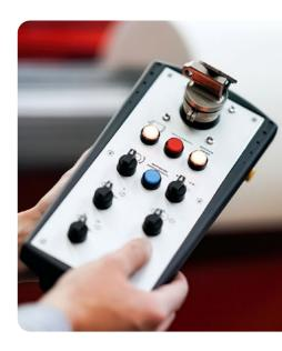
optimum handling of the machine both for setup, e.g. inserting the skiving block, and during operation, e.g. when changing the skiving speed or the film thickness. An extension of the control system, giving better repeatability of the film by product-related skiving and reeling programmes, is also possible.
