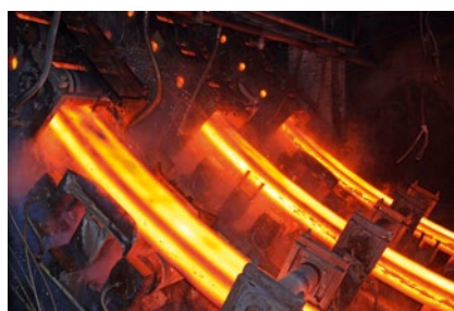
Installation de coulée continue
