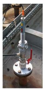
Pyrometer CellaTemp<sup>®</sup> PK with mounting
