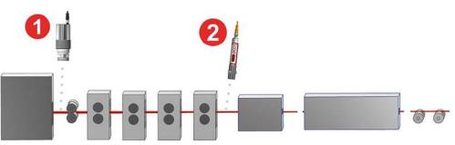
Temperature measuring points in the bar mill
