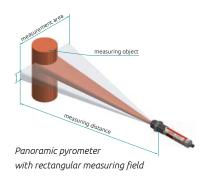
When measuring the temperature in the rolling stand, the rod can oscillate. The CellaTemp® PKL 63 two-colour pyrometer with panoramic optics is used to handle this demanding measuring task. The pyrometer has a rectangular measuring field. This is generated optically without moving components and is there-
