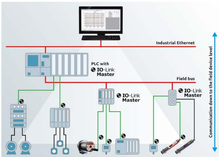
**Fig. 6** Integration of the pyrometer with IO-Link interface into the plant system control.
