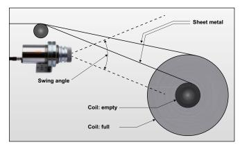
Fig. 5 Position of the roller gap at the coiler shifts in relation to the coil diameter.
