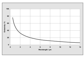
Fig. 1 The emissivity of metals decreases with an increasing wavelength.
