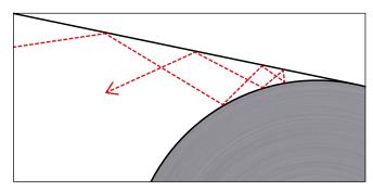
Fig. 4 Multiple reflection of the radiation between the sheet and the roller.
