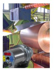
Fig. 8 Continuous-wave sensor pyrometers to measure temperatures from 75 °C upwards.
