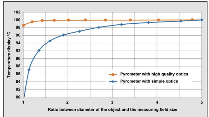
**Fig. 7** Changing temperature readings when the object size changes.
