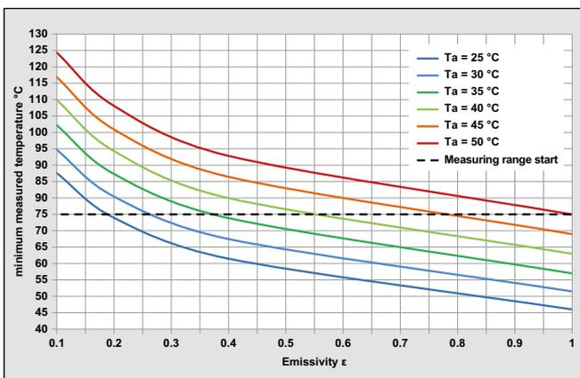
**Fig. 9** Minimum measuring temperature in relation to ambient temperature  $T_a$  and emissivity.
