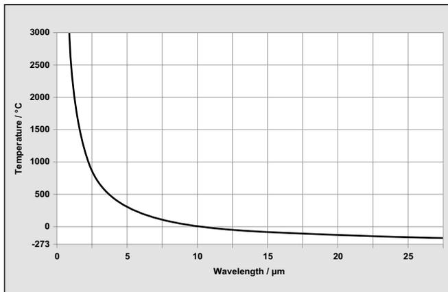
**Fig. 2** Wien's displacement law – relationship between the wavelength and the radiation maximum.
