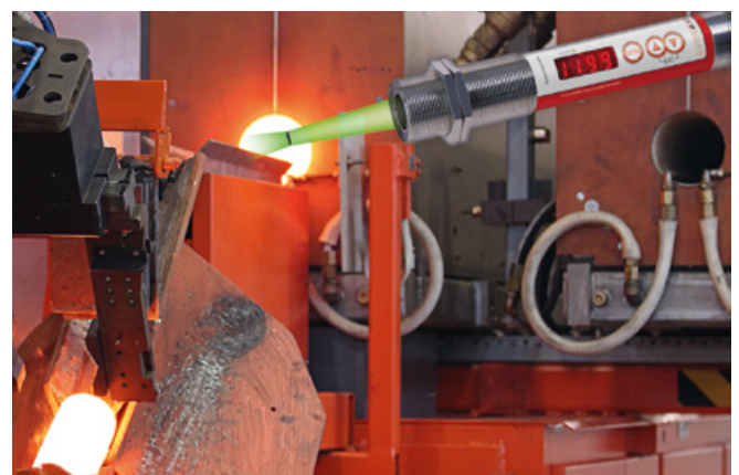
Fig. 2 Billets which are too cold or too hot can be rejected by switching outputs
