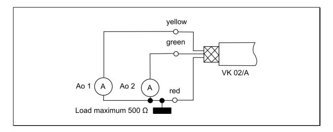
For all pyrometers of the PA Series the current outputs are short-circuitproof and share one ground connection via pin 8 of the connector. Each current output can be individually scaled and can be set either at the display or via interface.
