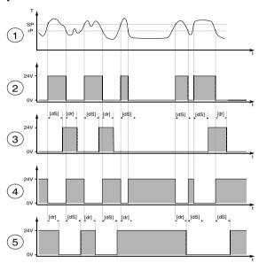
T = temperature P = P reset point P = P switch on delay P = P set point P = P switch off delay
