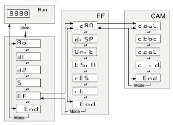
CAM Parameter and submenu only available at pyrometer with camera.
