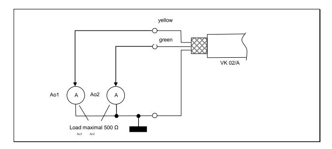
For all pyrometers of the PA Series the current outputs are short-circuitproof and share one ground connection via pin 8 of the connector. Each current output can be individually scaled and can be set either at the display or via interface.
