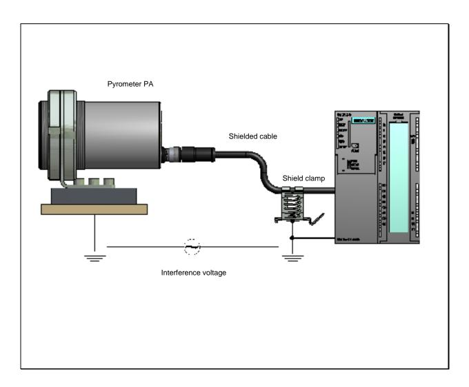
To avoid an equalising current, the pyrometer can be mounted electrically insulated. The shielding must be connected to the plant's earthing system.
