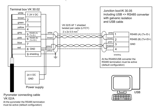
Moreover, use a converter with galvanic isolation (e.g. W&T 38211) to avoid problems with ground loops.
