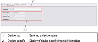
Under the category Identification there is the possibility to assign a name to this pyrometer in the field Device tag.
