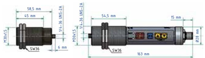
For the CellaSwitch PKS 21 the electronics are housed separately from the fibre optic sensor head. A fibre optic cable conducts the infrared radiation to the electronics assembly.
