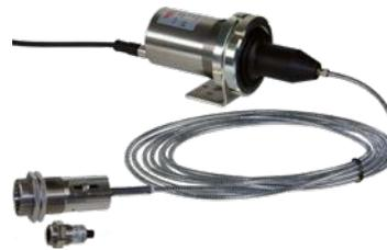
Limited space for installation or high ambient temperatures may require a separate optical sensor head and a fibre optic cable for the transmission of the infrared radiation to the evaluating unit. The sensor head can be used without cooling device up to ambient temperatures of 250 °C.
