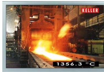
For optical adjustment, you have the option to select a CellaTemp PA 40 either with through-the-lens sighting, a laser or a colour camera. The target marker in the viewfinder or on the monitor defines the exact size and position of the measurement area.
