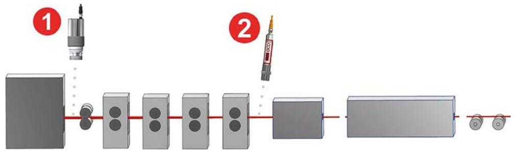
Temperature measuring points in the bar mill
