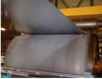
The measurement of metal sheets at low temperatures is still a challenging measuring task in the field of non-contact measurements due to the very low thermal radiation and the special radiation properties of metals.
