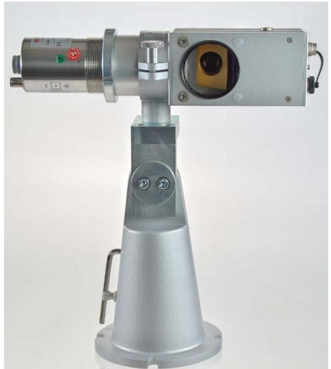
For the measurement, a pyrometer with laser sighting is recommended to detect the swivelling range and the speed and to adjust it optimally.
