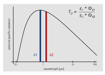
Pyrometers can be divided into single-colour and two-colour pyrometers.
