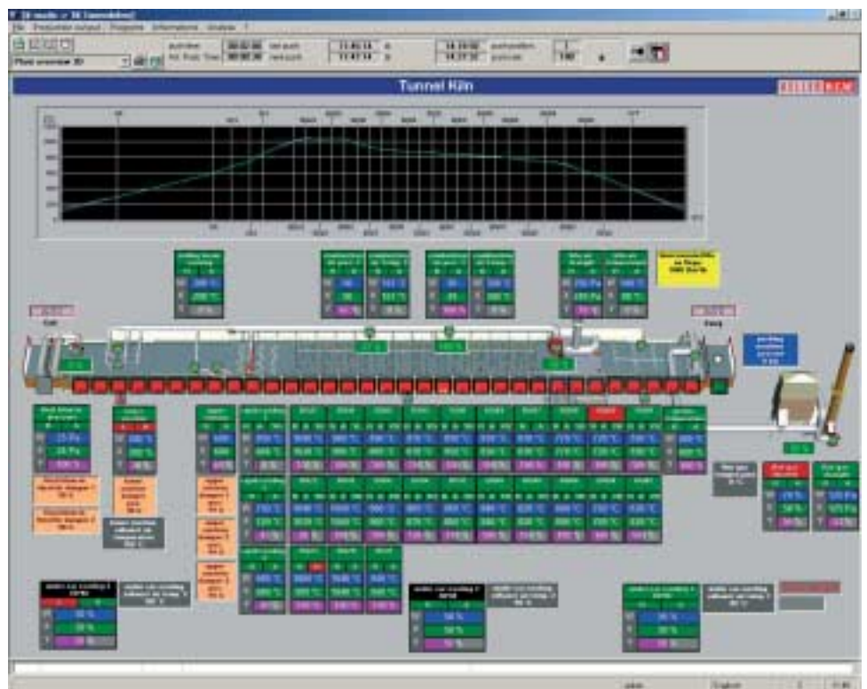
3D Plant overview with permanently shown firing curve
